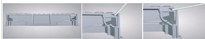
Particolari aggancio elastico- Details elastic system
